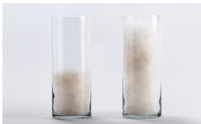
Both jars are filled with the same amount of down. The left jar shows non-treated down and the right jar shows NF5 treated down.
